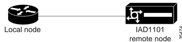
Before an inter node link can be provisioned, you must have an operational physical link between the two nodes. Both ends of the link must be in service and correctly provisioned before you can create an inter node link.
