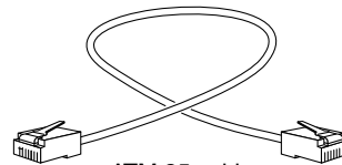
ATM 25 cable (green, RJ-45 to RJ-45) (Cisco 1401 router)
