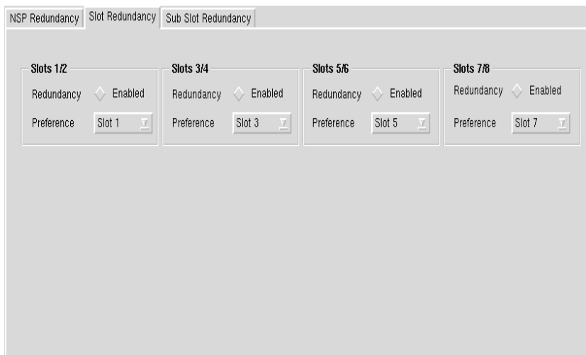
Figure 5-35 Cisco 6400 Redundancy Configuration Window (Slot Redundancy Tab)
