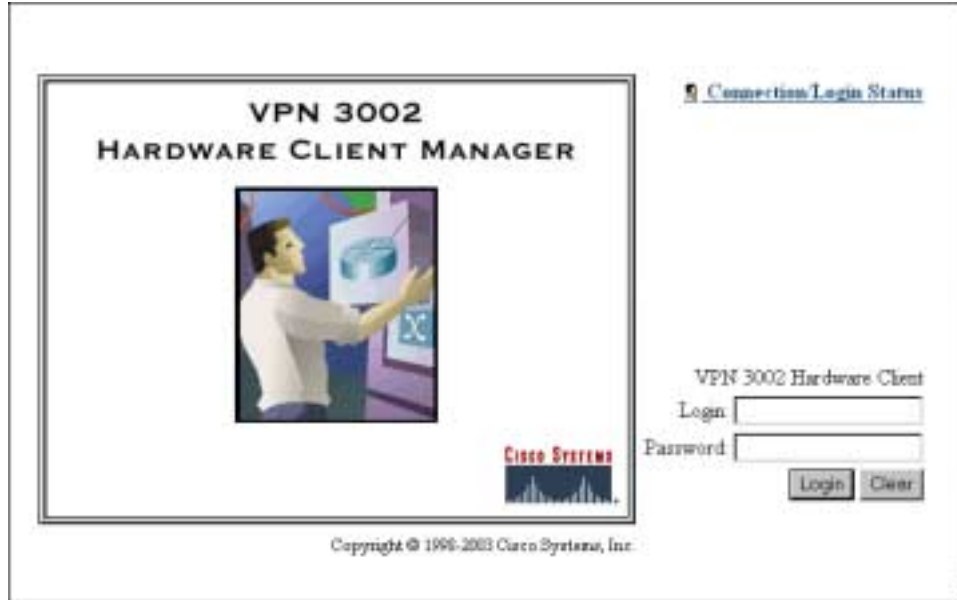
Figure 1-22 VPN 3002 Hardware Client Manager Login Screen Using HTTPS (Netscape)
