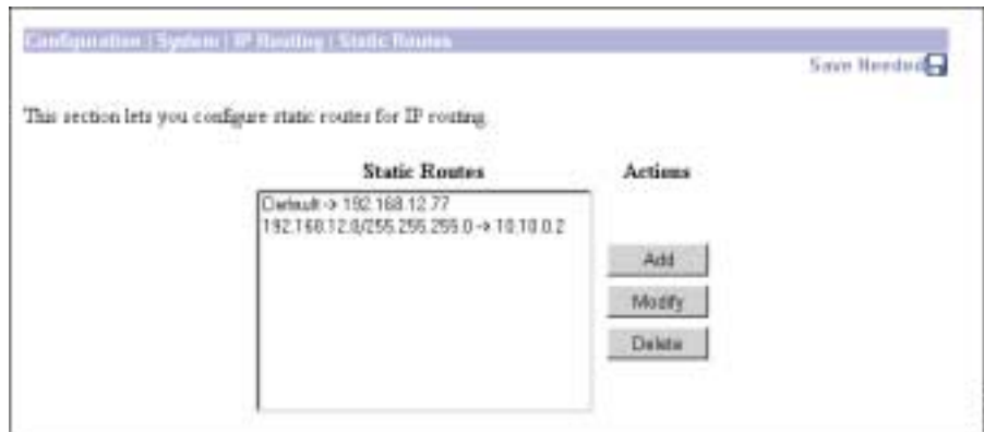
Figure 7-2 Configuration | System | IP Routing | Static Routes Screen
