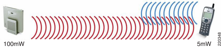
Figure 9-14 Client and AP Power Matching
